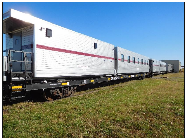
MOW boarding cars ready for shipment on the Industrial Structures spur.
