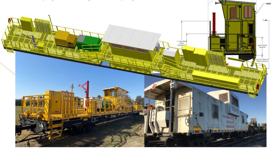
ISI (Industrial Structures Inc.) designed and manufactured a car that will replace the caboose's that a major rail operator has used for years to support their MOW crews delivering new rail and picking up the old rail.
